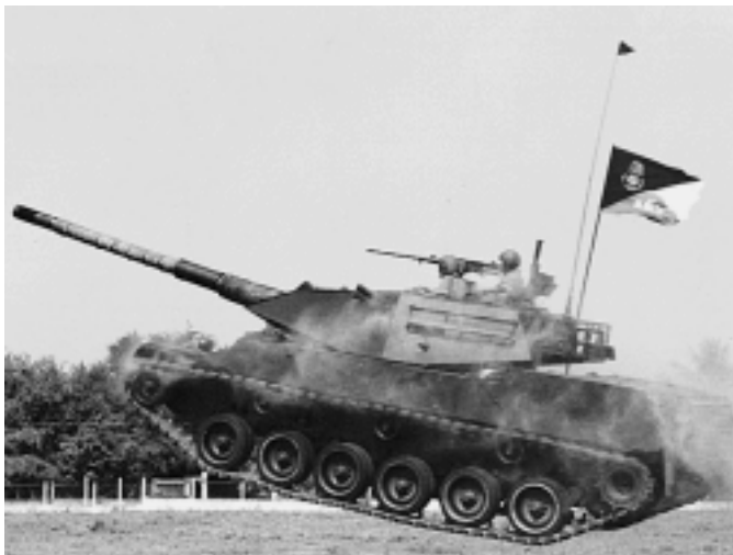
Figure 1. A Stingray Light Tank in service with the Royal Thai Army employing ceramic appliqué armour. Reproduced with permission from Jane's Information Group.
