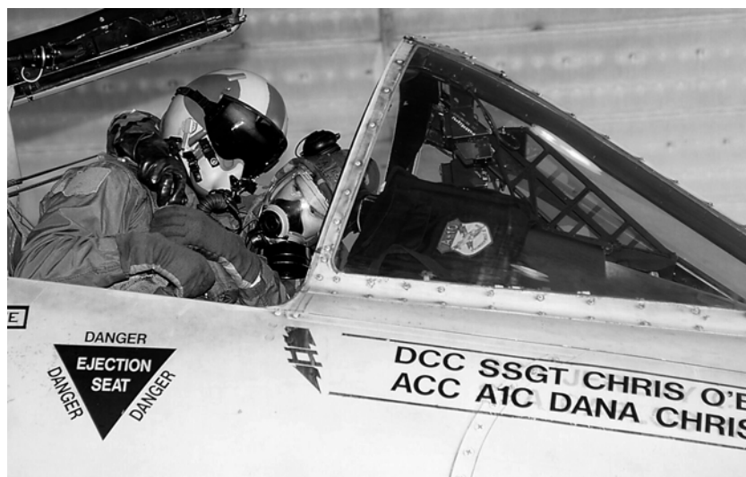
Figure 1-6. Ejection system warning markings on an A-10 Thunderbolt (photo courtesy of the United States Air Force).
