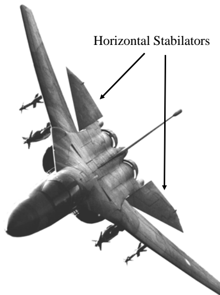
Figure 1-3. Horizontal stabilators on the F-111. (© Royal Australian Air Force).
