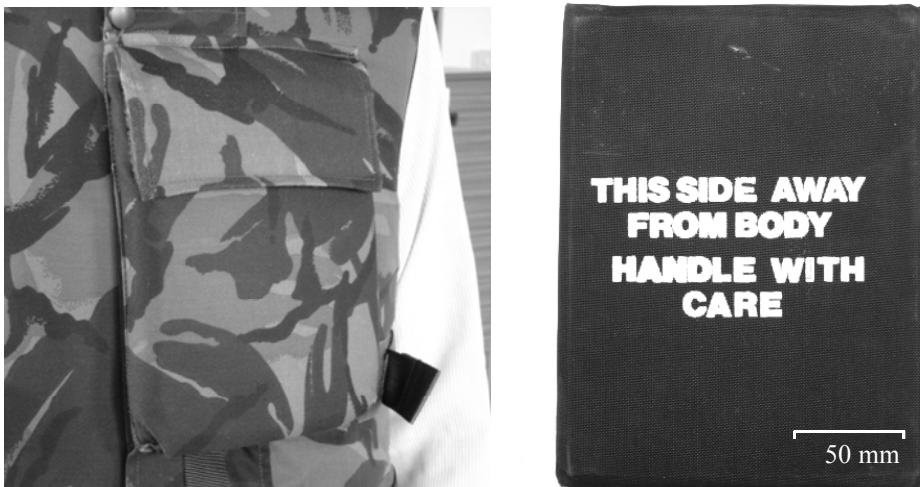
Figure 1-5: Combat Body Armour (CBA) showing the pocket for the ceramic plate insert (left) and a typical ceramic plate insert (right).
